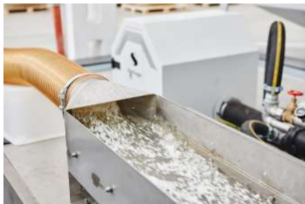
Detail regranulační linky Re-granulating line – detail
